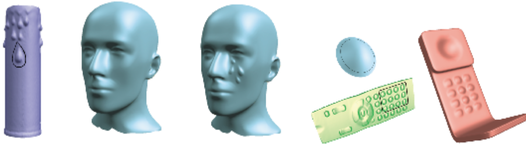
Figure 13: Left: details from a scanned candle pasted on the mannequin head. Right: features of different scales from other models added to a phone model.
